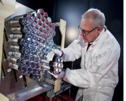
Inserting a read-out module into the prototype of the NectarCAM mini-camera in a darkroom. This large-scale structure (16 m long, 4.55 m high and 4.80 m wide) was designed to test, standardise and calibrate each of the camera's modules. © L.Godart/CEA
