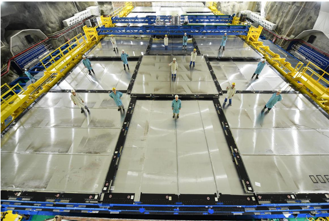
The Top Tracker. The Top tracker is a planar detector placed above the JUNO sphere. It identifies stray particles coming from the surface that can leave misleading traces in the detector. The Top Tracker is one of the main hardware contributions of the CNRS to the construction of JUNO. © JUNO Collaboration
