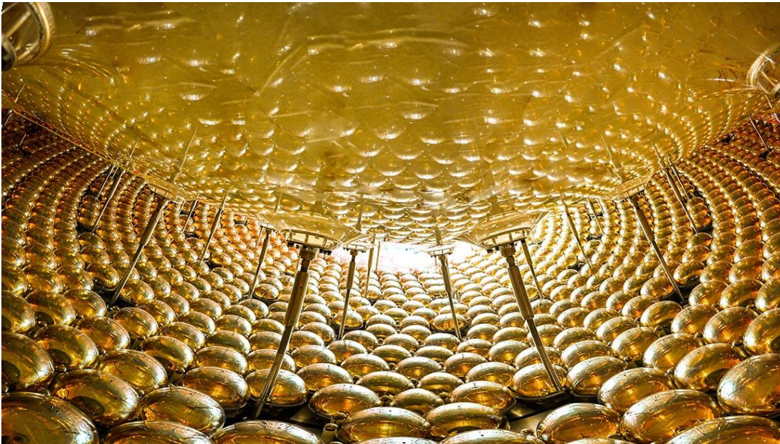
Photomultipliers monitoring the sphere filled with liquid scintillator. 43,212 photomultipliers of two types monitor light emission inside the JUNO detection sphere: large ones, which are clearly visible, and small ones interspersed between them. © JUNO Collaboration
