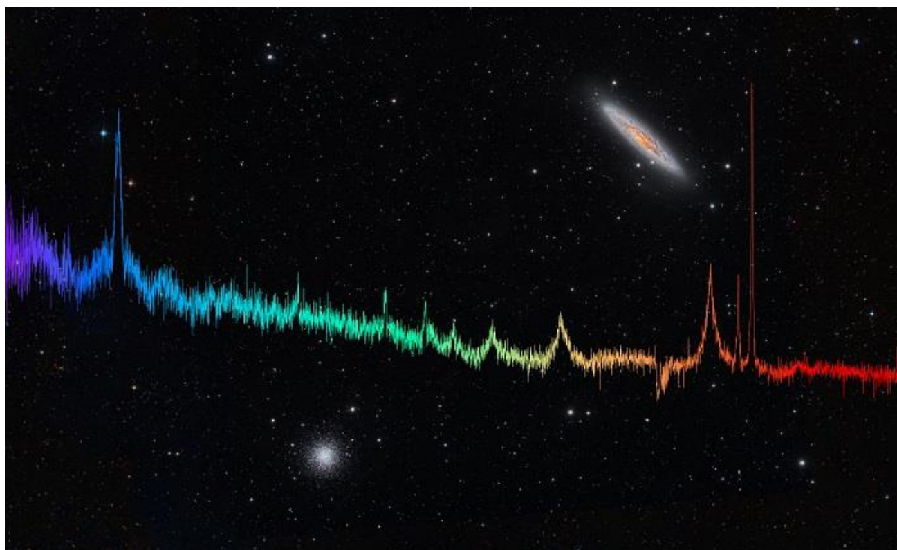
Figure 5: One of the over 2,000 spectra from 4MOST's first light, superimposed on the area of sky where it came from. Measured by pointing an optical fibre at a galaxy in the background, this spectrum reveals the typical shape of an active galactic nucleus (AGN), which indicates the presence of a supermassive black hole. Image: Roelof de Jong / AIP; Jens-Kristian Krogager / CRAL; Background image: Harshwardhan Pathak / Telescope Live
