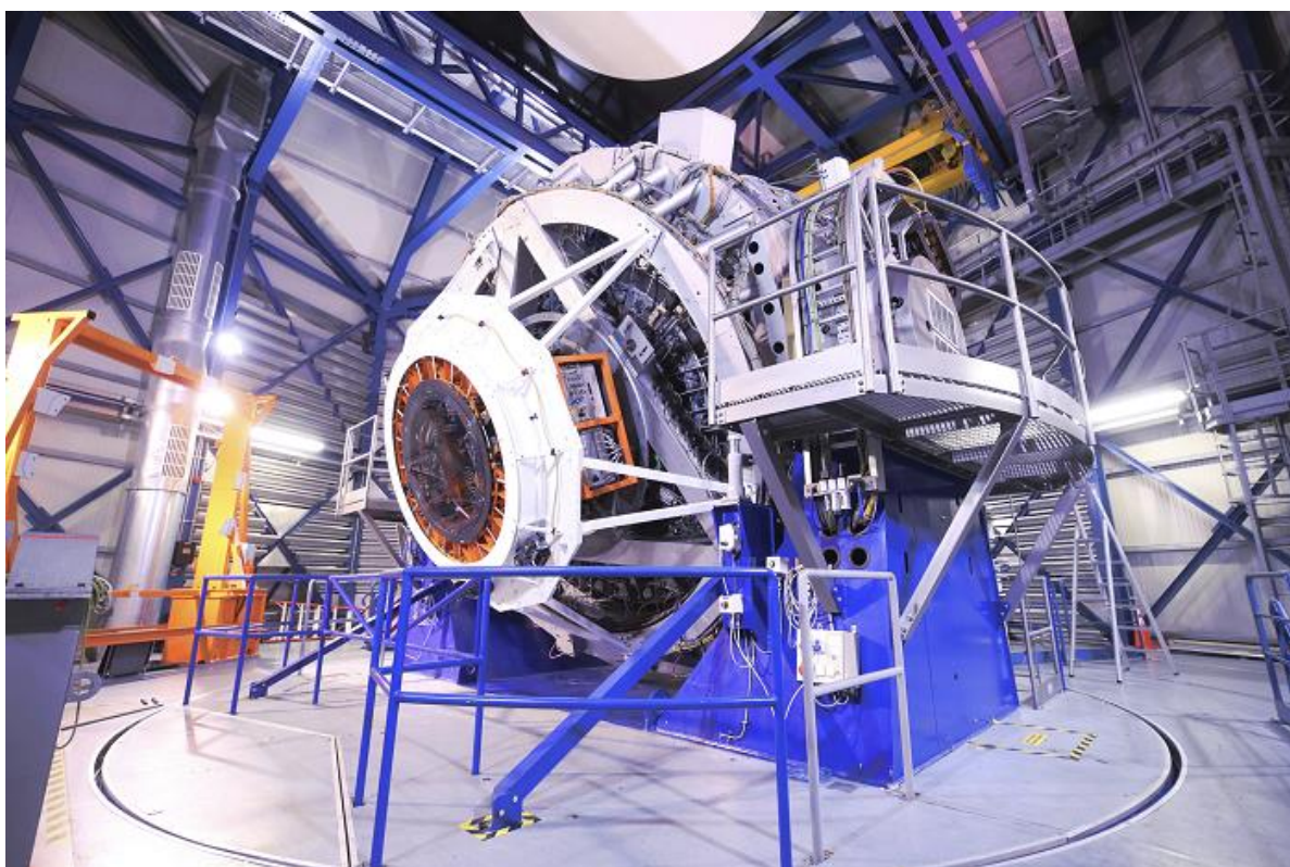
Figure 1: The Visible and Infrared Survey Telescope for Astronomy (VISTA) on which the 4MOST instrument is mounted. Image: Allar Saviauk / AIP
